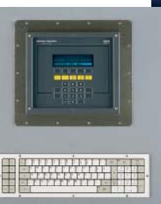
Speed data entry to the WI-130 Indicator with one of three optional alpha-numeric keyboards: the StanKey for normal settings, the TufKey 1 with spill resistent key membrane, and the TufKey 2 panel-mount version. One-year warranty applies.
