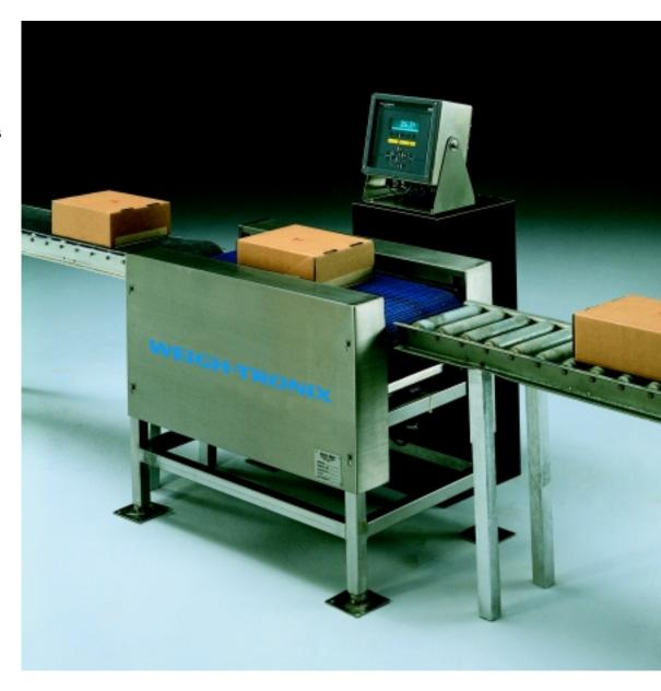
The Weigh-Tronix conveyor scale is a freestanding, self-contained and self-powered, flat-belt weighing system that can be incorporated into new or existing production facilities. The scale operates while the conveyor is in motion and is intended for the weighing of individual boxes, cartons, cans or unpackaged products such as large cuts of meat. It is ideally suited to checkweighing, straight weighing and weight accumulation operations.
