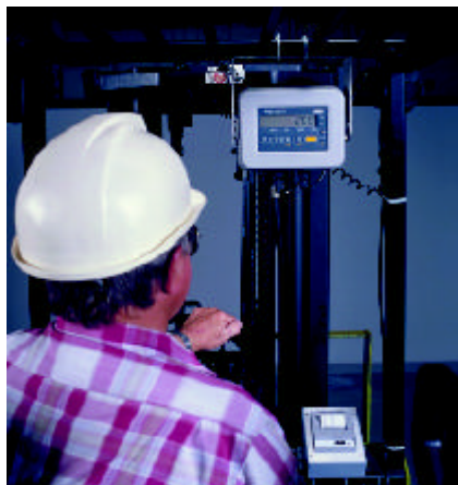
The WI-125 indicator linked with a WP-233 printer can provide an automatic hard copy of weight data.
