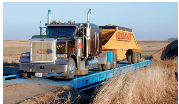
70' scale: three 23' 4" modules and eight weigh bars
